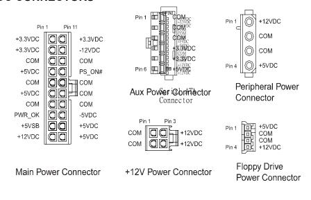
Typical ATX and ATX12V Power Supply Connectors (Pin-side view, not to scale)
